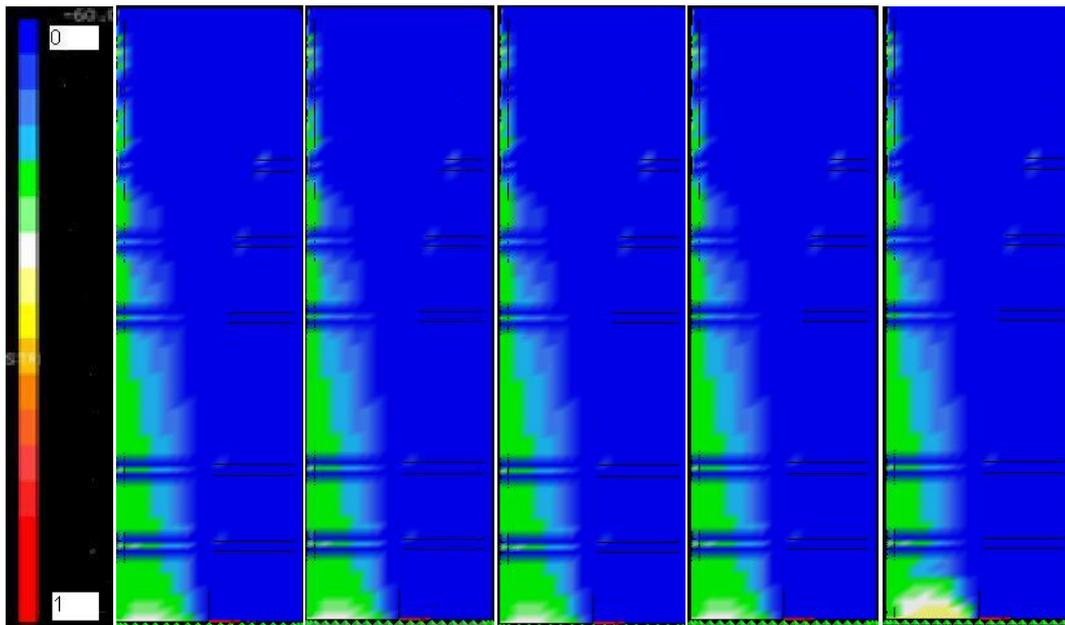
**Figure 6. Evolution of Triaxiality Index at 24%, 47%, 71%, 95%, and 100% of failure load**
