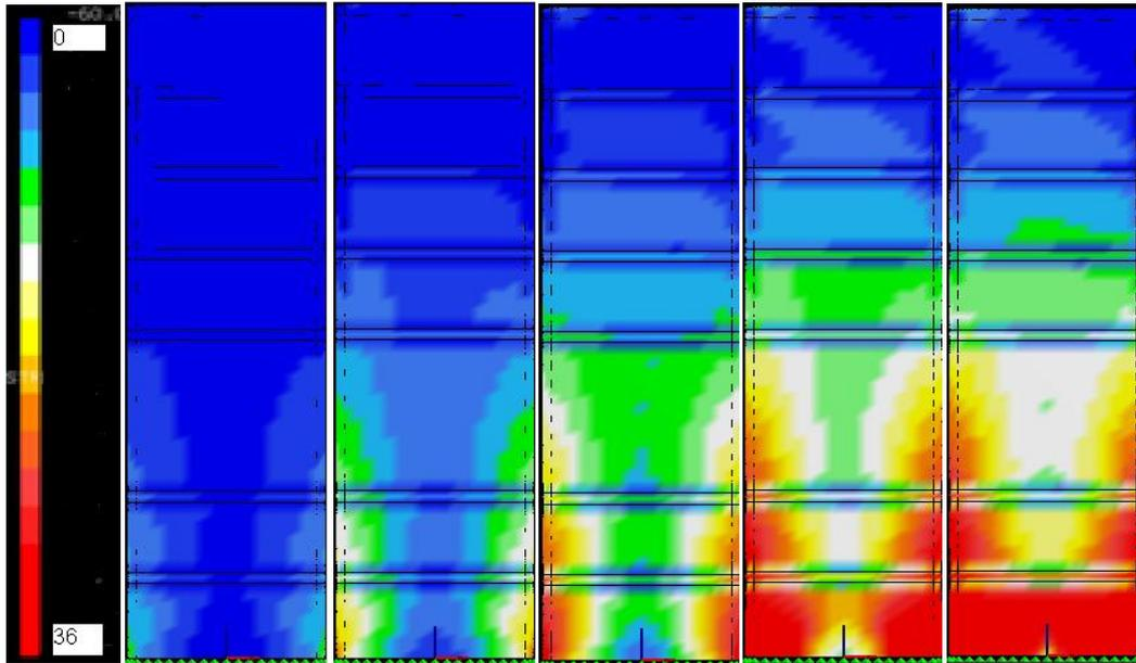
**Figure 5. Evolution of Von Mises stresses at 24%, 47%, 71%, 95%, and 100% of failure load**
