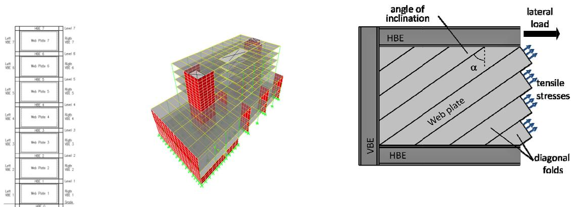
**Figure 2. (a) An elevation view of typical Steel plate shear (b) Completed building with special moment frames the traditional Reinforced Concrete shear wall, and (c) SPSW Tension Field**
