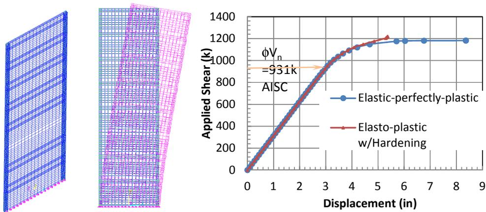
**Figure 4. (a) Finite Element Mesh, (b) Deformed at failure load, and (c) Applied Shear vs Lateral Displacement**
