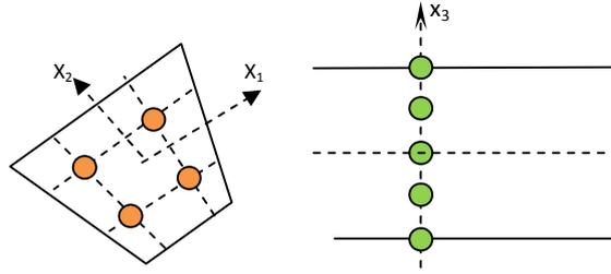
**Figure 3. Shell integration points: 1-2 axes (2x2 Gauss points), Axel 3 (5 Gauss-Lobatto points)**
