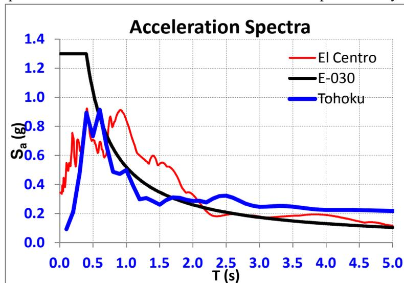
Figure 1. Strong ground motion Tohoku and corresponding Spectrum
